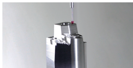
02-Obtain Actual Position on the Machine
